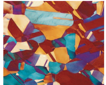
Annealed and cold drawn arsenical, phosphorus-deoxidized copper prepared using a four step process with MasterPrep® as the final polishing step and etched.
