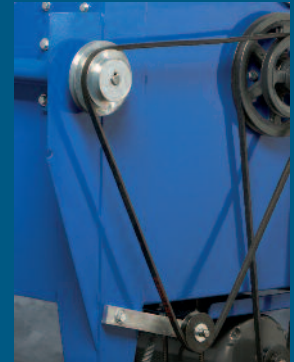
Step pulley allows the operator to change the feed rates.
