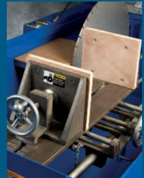
Rock Vise accepts a sample up to 17" (432mm) in size.
