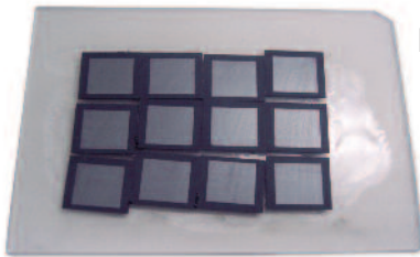
Multiple IC's are wax mounted on a glass slide
