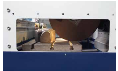
The windows on the sides can be removed in order to cut long samples.
