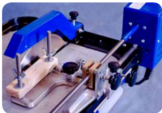
The Powerfeed mode moves specimen toward blade.
