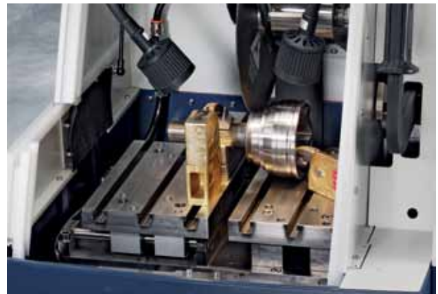
Speed vise and riser blocks provide vertical clamping forces for large and irregularly shaped samples.
