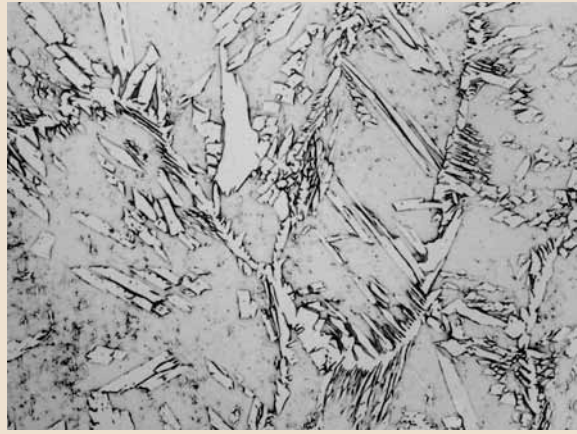
Duplex Stainless Steel, etched with Grossbeck's Reagent and prepared using: Apex DGD 30 \mu m, Apex DGD 6 \mu m, Apex DGD 3 \mu m, and ChemoMet ® with MasterPrep ® , 50X.
