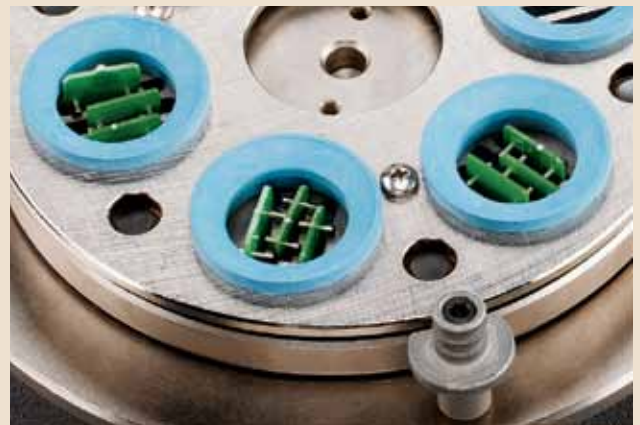
Printed wiring board coupons ready for molding compound in the PWB Met™ Small Hole Accessory.
