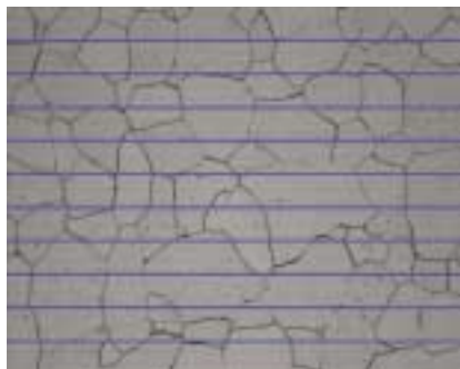
An illustration of the Heyn Lineal Intercept Procedure adapted for automated image analysis use.
