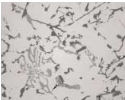
As polished type 332 cast Al with phosphorous.
