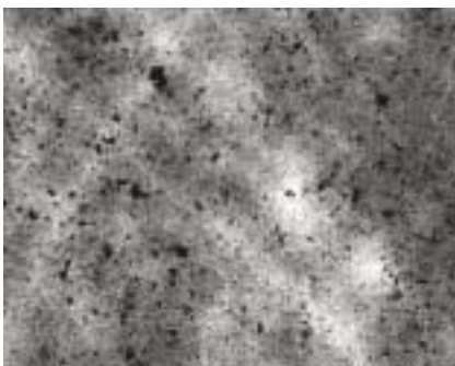
Debris from transmission fluid captured with filter paper.
