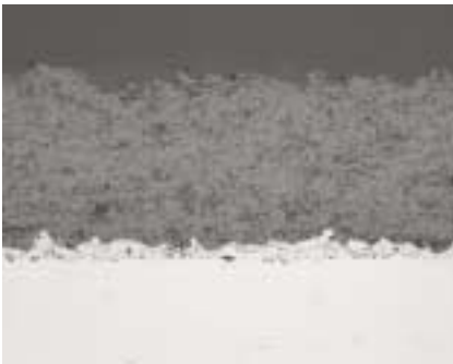
As polished 8% yttria stabilized zirconia thermally sprayed coating with a NiCrAl bond coat.
