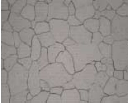
Low carbon steel alloy etched with picral to reveal the grain boundaries.
