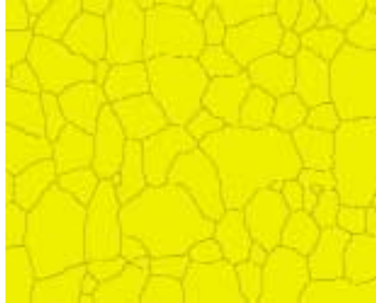
After detecting the grains, the boundaries are thinned to be only one pixel wide.
