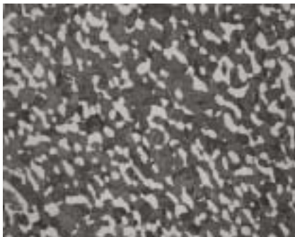
Microstructure of wrought Ti-8%Al – 1%Mo-1%V etched with Kroll's reagent.
