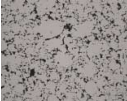
As polished ferrous gear formed by powder metallurgy processes.
